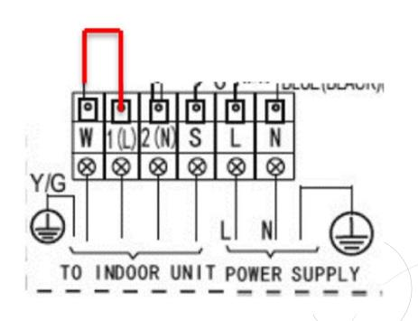
For instances where a 4 core interconnecting is to be used we can bypass the 1W standby relay and power the condenser directly from the mains supply
