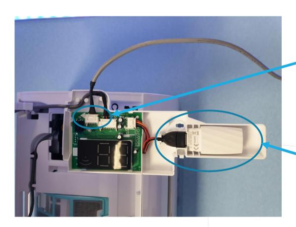
**CN2** – KJR29B controller uses an adapter cable to connect to the wall mounted units
